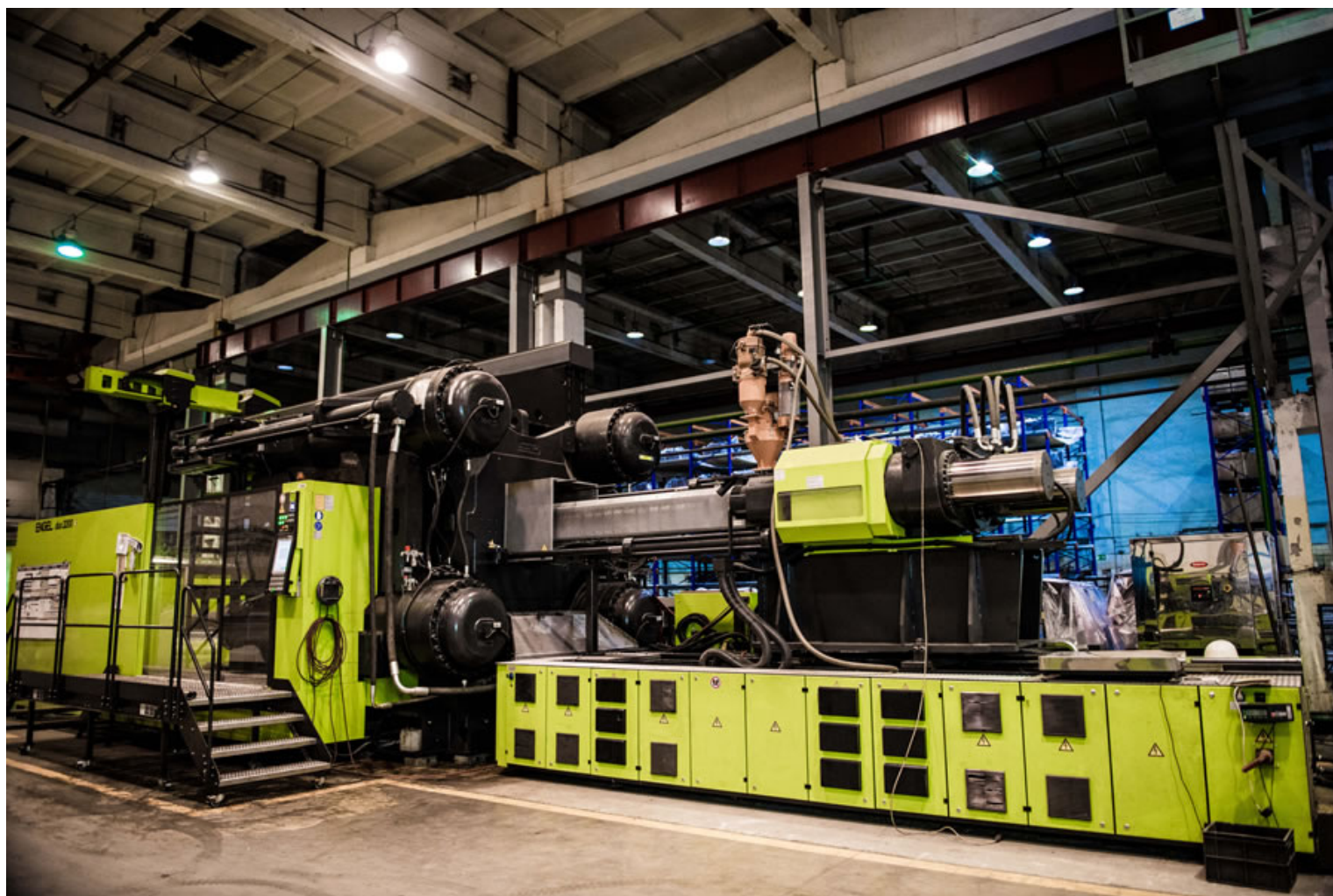
ENGEL duo 3200 (injection moulding machine for large parts).
