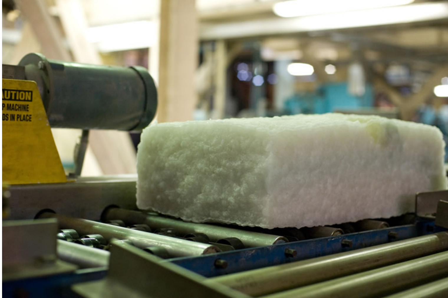
A briquette of high-viscosity polybutadiene rubber (BR-ND HV).
