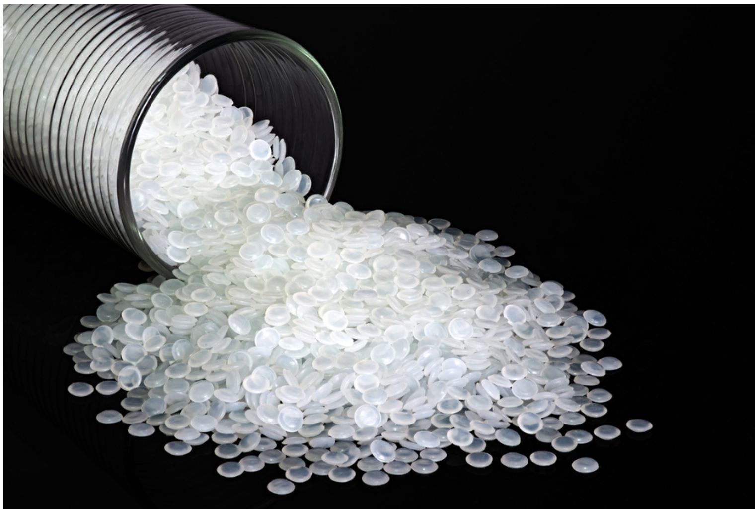
PP granules resulting from the mechanical recycling of polymer waste. Still, chemical recycling holds the biggest potential for SIBUR.
