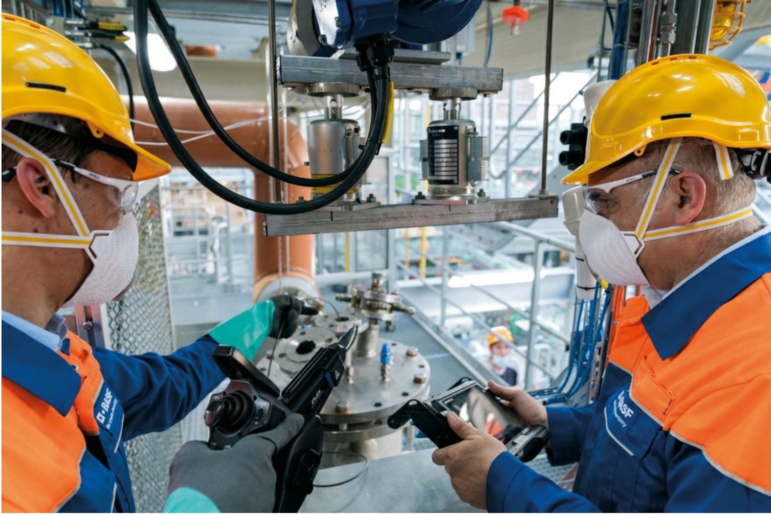
Zero-carbon methane pyrolysis technology used to produce hydrogen from natural gas is being tested at Ludwigshafen.
