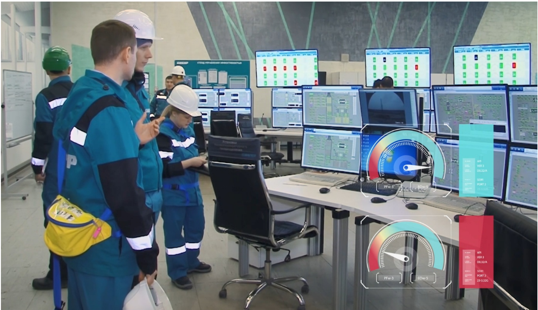
The decision support system visualises the economic performance of the current operating mode and helps the operator to make production process more efficient.
