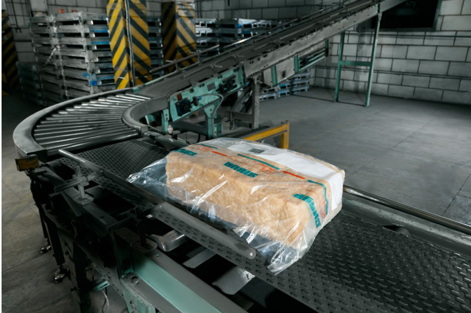
A briquette of a butadiene rubber (BR) grade on the conveyor belt at Voronezhsintezkauchuk.
