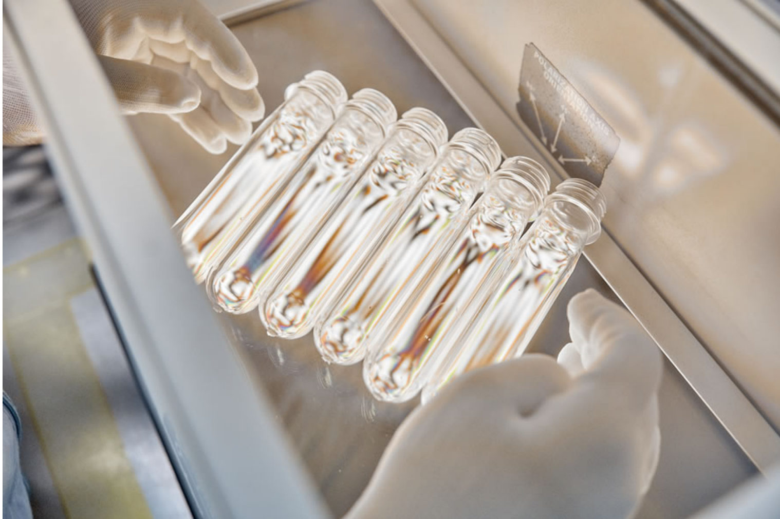
The production of PET preforms.
