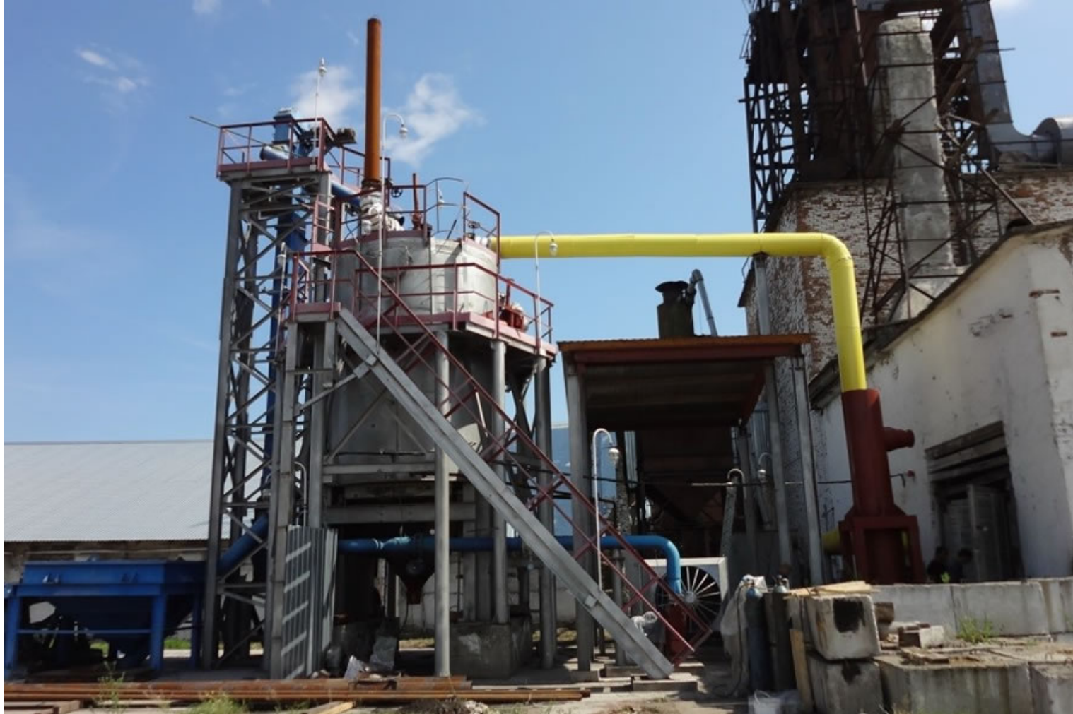
Equipment to produce combustible gas from coal for drying grain, Balakhta, Krasnoyarsk Territory Source: termokoks.ru.
